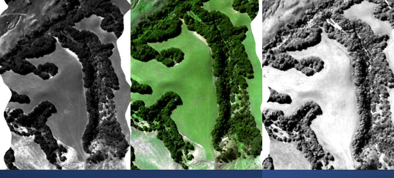
Distinguishing features Pasture and soil in different wavelengths Distinguishing features poplar tree and pasture in different wavelengths
